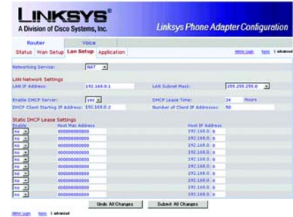
Figure 6-6: Router - LAN Setup Screen
