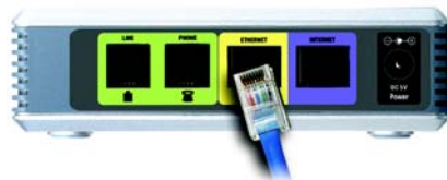
Figure 4-3: Connect a PC
