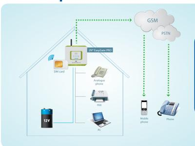
You can connect an analogue phone or PBX to get voice connection. A PC connected to a USB port can access the Internet and send/receive SMS messages.
