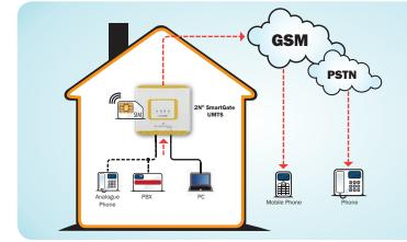
You can connect an analogue phone or PBX to get voice connection. A PC connected to a USB port can access the Internet, and the sending/receiving of SMS messages can be done using the SMS program. The 2N<sup>®</sup> SmartGate UMTS can be used in areas where a fixed line is not available, or as an alternative for persons/companies that no longer want to use fixed lines.
