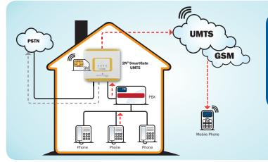
When you connect the 2N<sup>®</sup> SmartGate UMTS between the PBX and the network, the routing service can be performed by the gateway without programming the PBX. You will therefore save one of the PBX ports and all calls to mobiles will still be routed via 2N gateways. In this con-figuration, it's easy to implement Mobility Extension when nobody is online in the company. ۲
