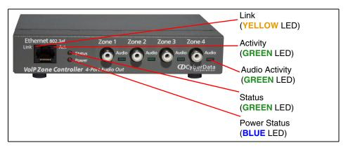
3.2. The round, **BLUE Power Status** LED on the front of the Zone Controller comes on indicating that the power is on.
