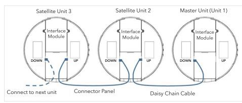
Every Quattro3 comes with the built-in ability to connect to other Quattro3s (up to 15 units). This feature enables you to provide coverage for larger spaces using a chain of Q3s.
