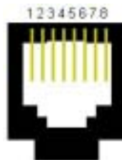
Figure 2-2 10/100 BASE-T Ethernet Port Pin Order
