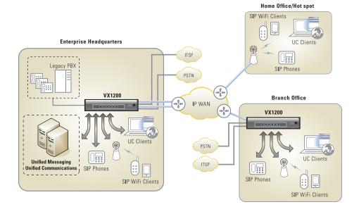
ENTERPRISE-CLASS INTEGRATION OF UNIFIED COMMUNICATIONS WITH TELECOM INFRASTRUCTURE: NET's VX Series and Tenor Series Media Gateways provide full connectivity between Unified Communications and Telecom infrastructure. NET's portfolio meets the Media Gateway requirements for UC deployments for large to small enterprises for their headquarters and branch office locations.
