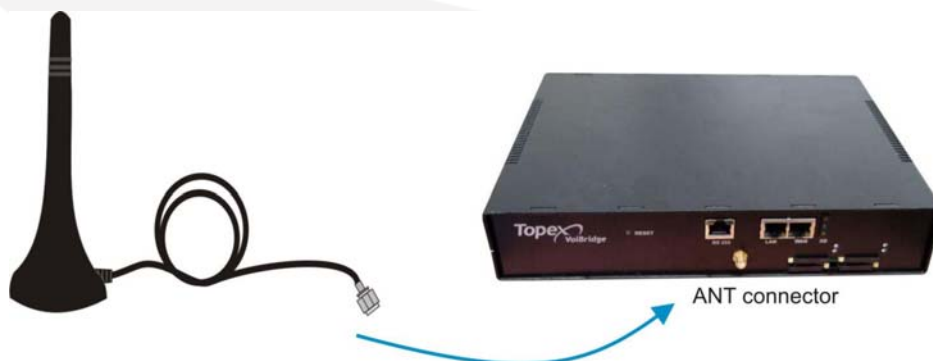
Figure 13 – Mobile antenna connection
