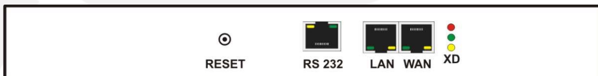
Figure 6 – PGVoIP card connectors
