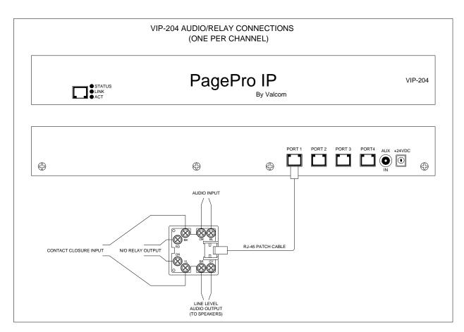
**AUX Input:** Local audio may be input via the rear panel RCA jack. Nominal input impedance is 600 Ohms. Connect any compatible audio source using an RCA patch cable. Audio supplied through the rear panel RCA jack broadcasts to all Audio Outs whenever they are idle. This is typically used for background music.
